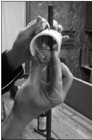
Temperature sensor (HOBO TidbiT v2) and protective housing that BRWA has deployed at several stream sites near the potential iron mine site east of Mellen.
