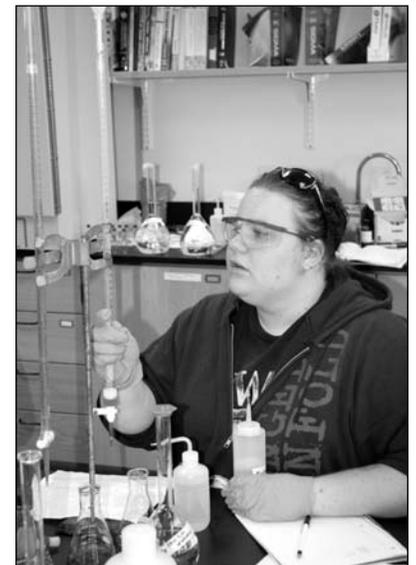
*Northland Student Margot Seiler carefully reads the buret during the alkalinity titration test.*
