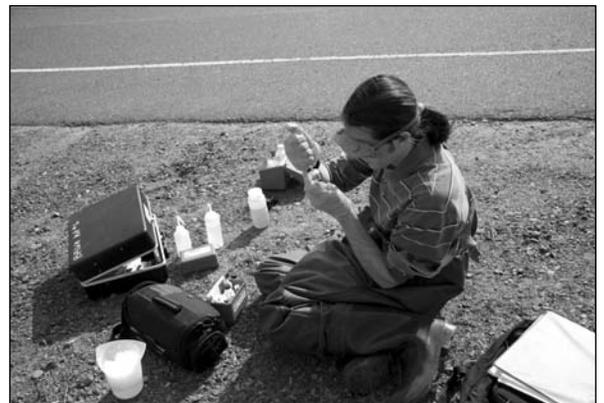
**Northland Student James Tilley titrates the water sample to find the chloride level. Each kit is brought into the field and used on site.**
